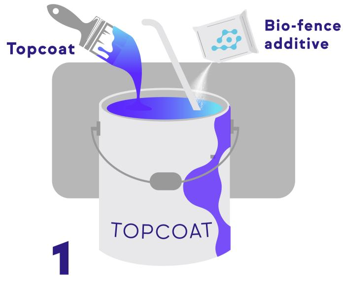
Add the Bio-fence additive to the paint / topcoat.
